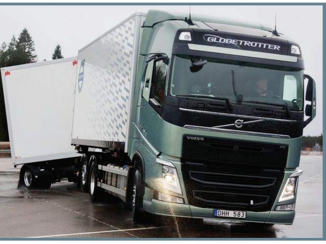
Clockwise from main picture: Volvo Trucks' Stretch Brake system, developed to reduce the risk of jack-knifing and trailer instability
